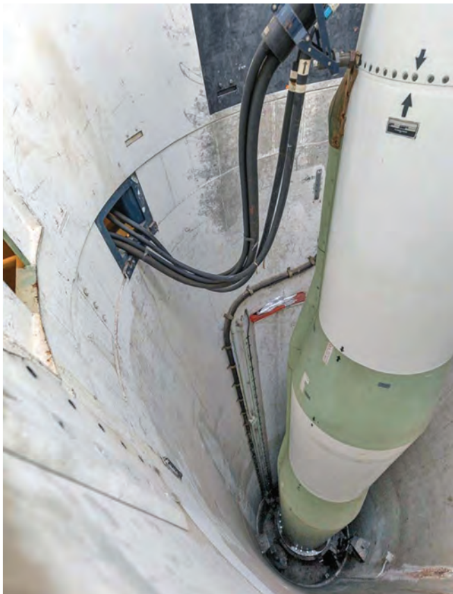
A view down the missile silo showing all of the rocket's three stages along with the shock isolated thrust mount on which the missile sits. Photo Chris Howells
